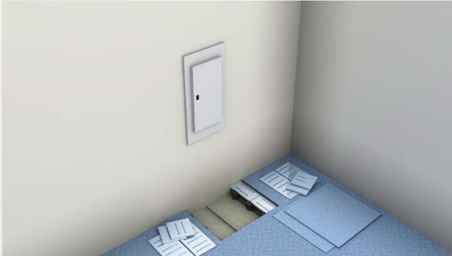
Homerun Cable to Electrical Panel - (3 circuits each)
