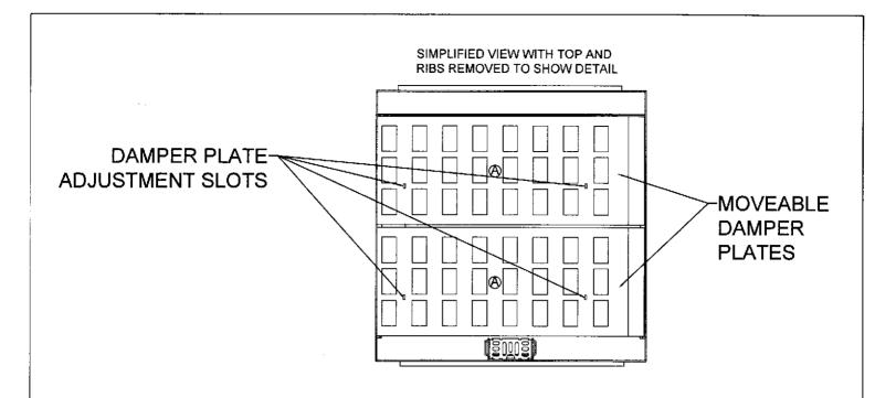
DAMPER PLATES (2) ARE EASILY ADJUSTED THROUGH SURFACE OF GRATE WITH A FLAT HEAD SCREWDRIVER PASSED THROUGH A SLOT OPENING AND INTO THE DAMPER SLOT, THEN "TILTED" ONE WAY OR THE OTHER TO INCREASE OR DECREASE AIR (CFM) VOLUME.
